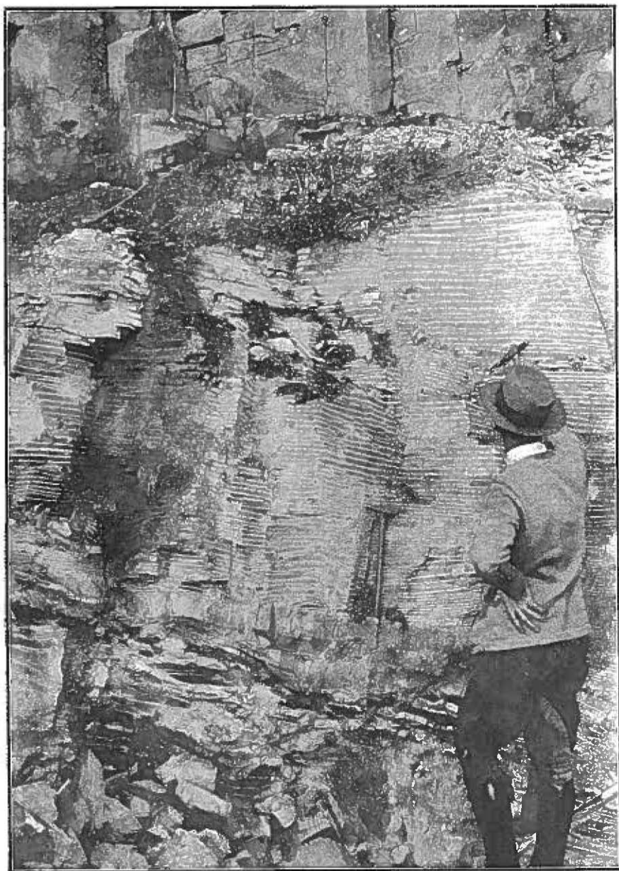
PLATE XI.— New Amianthus Mines , near Kaapsche Hoop (Barberton District) showing the characteristic association of countless parallel chrysotile seams.
